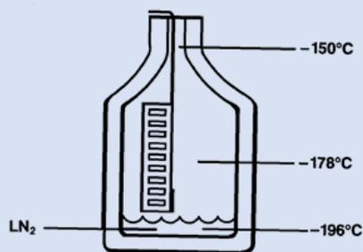
Sample tubes have been known to explode when removed from liquid nitrogen storage due to seepage of liquid nitrogen into the tube which expands rapidly on warming. This not only represents a significant risk injury but potentially also an infection risk (depending on the contents of the tube).
