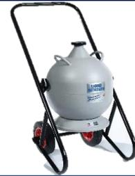
**Pressurised Dewar's** - larger quantities (up to 500 litres) are generally held in transportable pressurised cylinders. They are fitted with safety devices to allow them to vent excess pressure.
